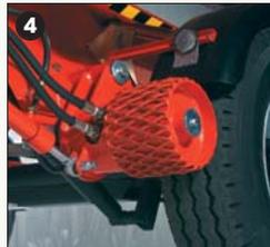
**4.** Hydraulic drive wheels for ease of movement.
